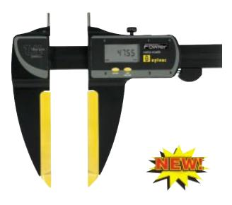
Fowler/Sylvac's new lightweight heavy-duty electronic digital calipers include sizes up to 60"(1500mm) and resolution of .0005"(.01mm). This has been achieved by designing a well-balanced instrument utilizing state-of-the-art material technology. Functional parts are made of the latest wear-resistant materials. Hollow section aluminum beam reinforced by two stainless steel guides. This system assures perfect guidance and protects the beam against shocks.
