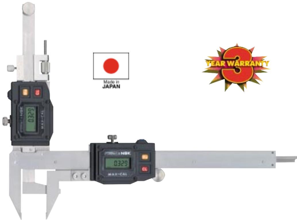
The Gear Tooth Max-Cal is used for the testing of gear teeth. The vertical scale measures the depth of teeth from the top to the pitch line, and the horizontal scale measures the thickness of teeth in the pitch line.
