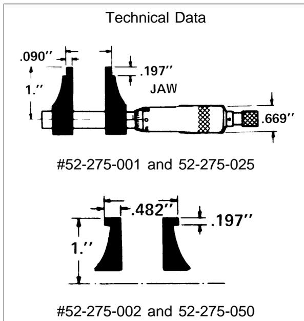
With Fowler Inside Micrometer Calipers, you are assured of smooth operation and stabilized uniform accuracy. The frame is specially designed to enable the micrometer to provide extremely accurate small internal measurements.
