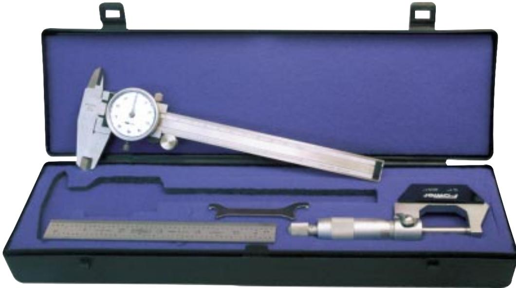
The Fowler Toolmaker Universal Measuring Set is ideal for the apprentice to start adding to his tool inventory. Set consists of "One-Rev" Dial Caliper, a 0-1" Micrometer and a Flexible 6" Rule. This set is also recommended for school shops and training programs for future tool-makers and machinists.
