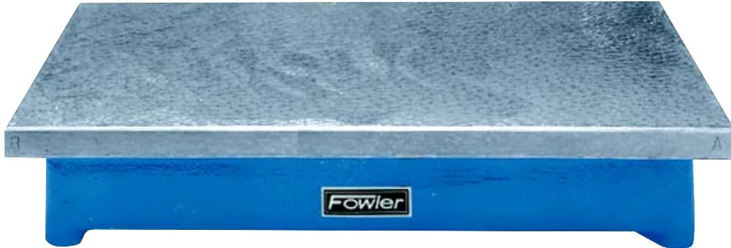
Cast Iron Surface Plates are made from close-grained cast iron, heat treated and stress relieved to a hardness of 170—220 BHN.
