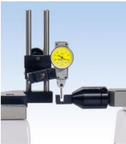
▲ checking of lever (test) dial indicators using 54-197-115
