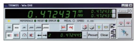
Trimos-Win DHI software for all required measuring functions and connection of a gage inspection and management system
