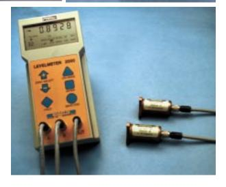
The instrument has two individual measuring channels. The display can be adjusted for:
