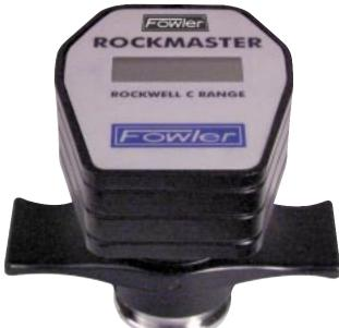
Fowler's Rockmaster is a robust, superbly finished portable, digital hardness tester with direct readout, requiring minimal maintenance. An ideal tool for inspectors and quality control engineers for on-site checking, it is generally used in a vertical position but may be used in almost any direction even on circular sections—without affecting accuracy.
