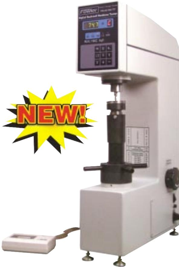
Fowler's New Digital Rockwell hardness tester offers fully automatic operation and output.
