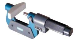
This micrometer was manufactured to measure items with staggered teeth, such as side milling cutters and saws. In place of the usual anvil, a rectangular pad has been mounted that bridges the gap between the adjacent measurement surfaces. Sizes over 1"/25mm include a standard.
