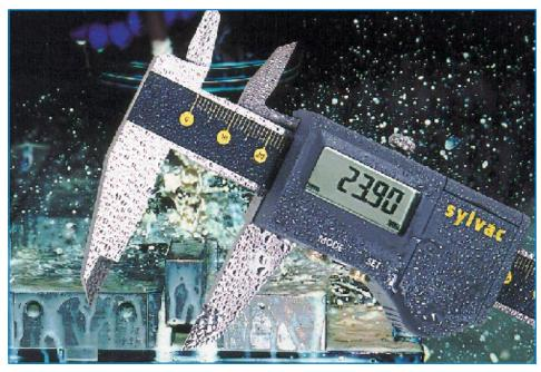
which in turn inducts voltages in the other windings. Sampling these voltages and repeating the process generates a waveform ultimately yielding the position. Even though the pulse current rises to about 200 milliamps, the caliper's average current consumption is kept below 50 microamps by the low pulse repetition rate.
