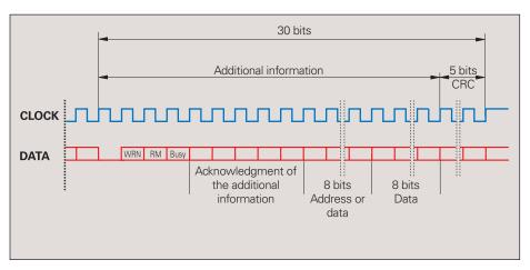
The additional data always The additional data can contain the following information: begin with: **Additional information 1** Additional information 2 Status data Warning—WRN Diagnosis Commutation Position value 2 Reference mark—RM Acceleration Parameter request—busy Memory parameters Limit position signals Acknowledgment of MRS-code acknowledgment additional information Test values Temperature
