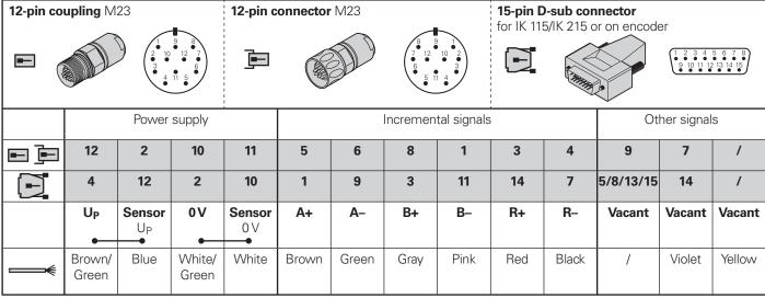
**Shield** on housing;  $U_P$  = Power supply voltage
