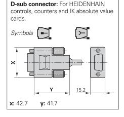
The pins on connectors are **numbered** in the direction opposite to those on couplings or flange socket, regardless of whether the contacts are
