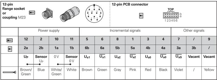
**Shield** on housing;  $U_P$  = Power supply voltage
