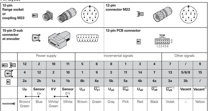
**Shield** on housing;  $U_P$  = Power supply voltage
