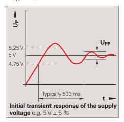
The values apply as measured at the encoder, i.e., without cable influences. The voltage can be monitored and adjusted with the device's sensor lines. If a controllable power supply is not available, the voltage drop can be halved by switching the sensor lines parallel to the corresponding power
