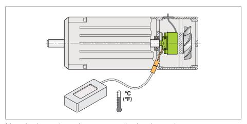
Measuring the actual operating temperature directly at the encoder
