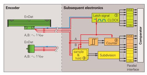
After power on and initial transmission of position values, two redundant position values are available in the subsequent electronics. Since encoders with EnDat interface guarantee a precise synchronization—regardless of cable length—of the serially transmitted absolute value with the incremental signals, the two
