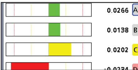
**Visual feedback** A highly visible, intuitive and familiar interface with standard color cues. Instantly informs operators of pass/fail performance details for critical part dimensions.
