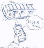
Simply set the diameter of a rotating shaft to make non-contact conveyor belt or other line speed measurements.
