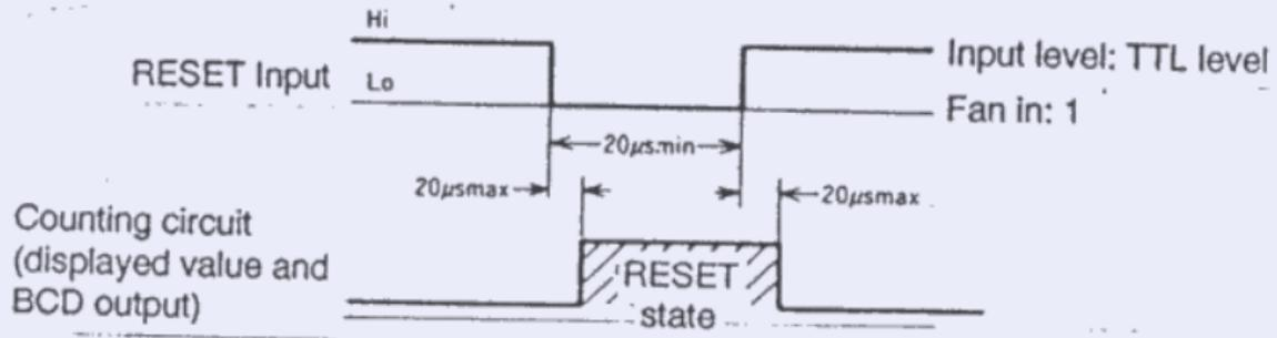
The RESET signal must have a pulse width of minimum 20  $\mu$ s. It takes up to 20  $\mu$ s from RESET signal input to RESET state and from RESET signal release to RESET state release, respectively.
