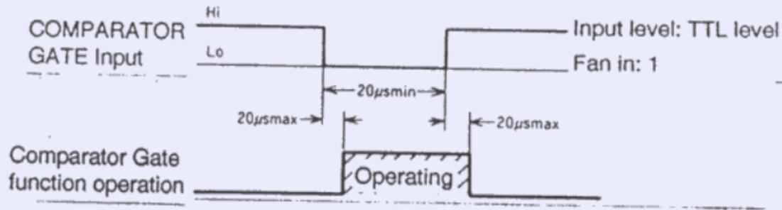
The COMPARATOR GATE signal must have a pulse width of minimum 20  $\mu$ s. It takes up to 20  $\mu$ s from COMPARATOR GATE signal input to its functional operation start and from COMPARATOR GATE signal release to function release, respectively.
