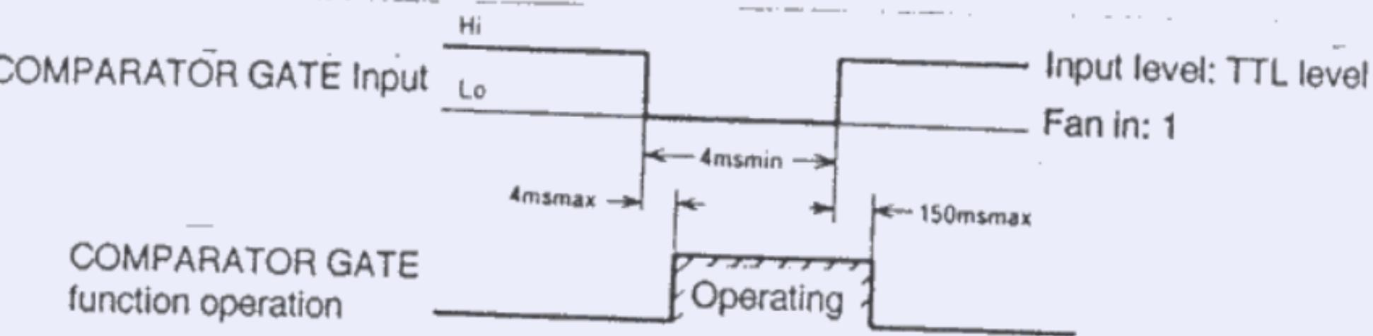
The COMPARATOR GATE signal must have a pulse width of minimum 4 ms. It takes up to 4 ms from COMPARATOR GATE signal input to its functional operation start. It takes up to 150 ms from COMPARATOR GATE signal release to functional release.
