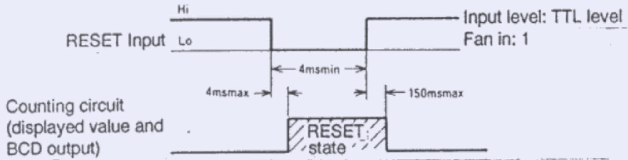
The RESET signal must have a pulse width of minimum 4 ms. It takes up to 4 ms from RESET signal input to RESET state. It takes up to 150 ms from RESET signal release to RESET state release.
