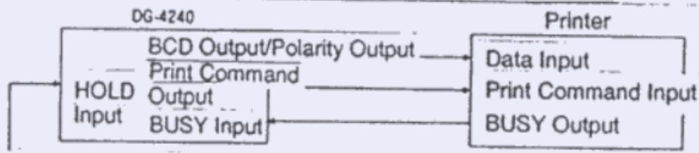
This timing chart shows that the printer is started at the rising of the print command signal. Retain the HOLD Input at the low level until the BUSY Input becomes the low level.
