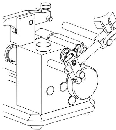
Figure 13. Back Stop Assembly (Rear view)
